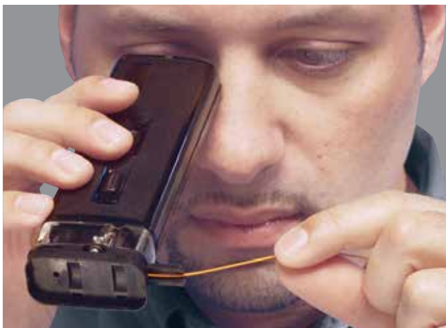
Example of microscope for visually checking the surfaces of the connectors and connector cleaning kit
